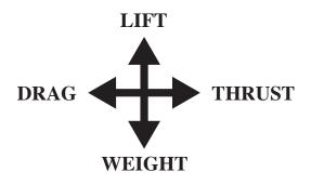
What really causes an airplane to fly? The answer is that four forces act upon an aircraft in flight, one acting up, one down, one forward, and one backward. *Lift* is the upward force generated by the wings, while the *weight* of the plane acts downward. The *thrust* of the engines propels the plane forward, while *drag* (think wind resistance) holds the plane back. Lift and thrust are positive forces for flight; weight and drag are negative forces.
